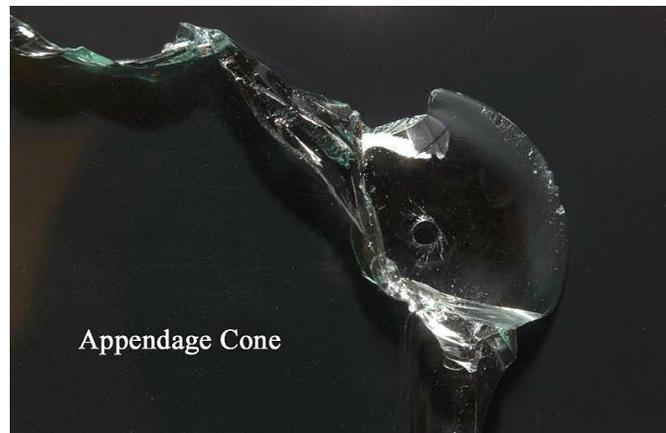
**Figure 2** *Appendage Cones are attached to overburden.*
