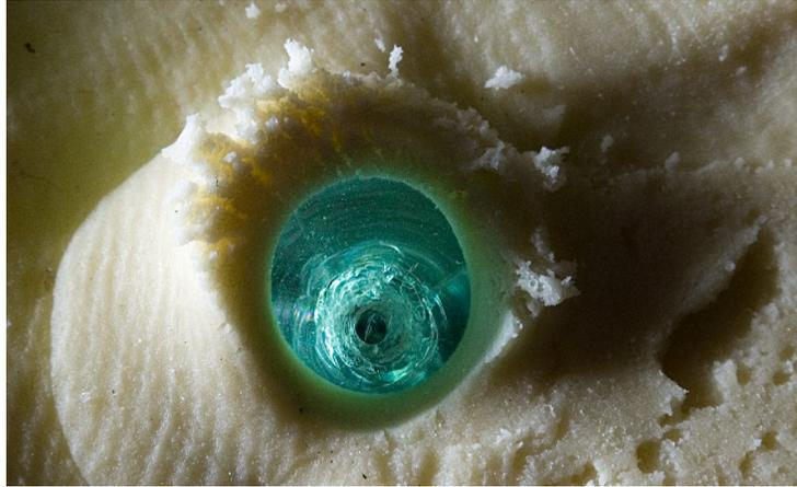
**Figure 10** A crater and sub-surface Hertzian cone. A combination of 5mm soda lime glass and a "crustal" coating of modeling clay. The crater was made by a 5mm steel projectile.
