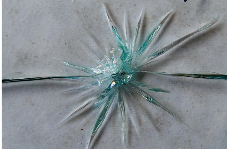
**Figure 38** An X or Star Fracture created when projectile bends target material creating a fracture from a lower plane or strata. The feature is sometimes call a Lotus Fracture due to parabolic, petal-like fractures from the main HC as seen above.
